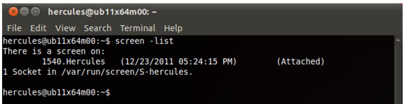
A terminal window titled 'hercules@ub11x64m00: ~' with a menu bar (File, Edit, View, Search, Terminal, Help). The terminal shows the command 'screen -list' being executed, resulting in the output 'There is a screen on: 1540.Hercules (12/23/2011 05:24:15 PM) (Attached) 1 Socket in /var/run/screen/S-hercules.'. The prompt returns to 'hercules@ub11x64m00:~\$'.
