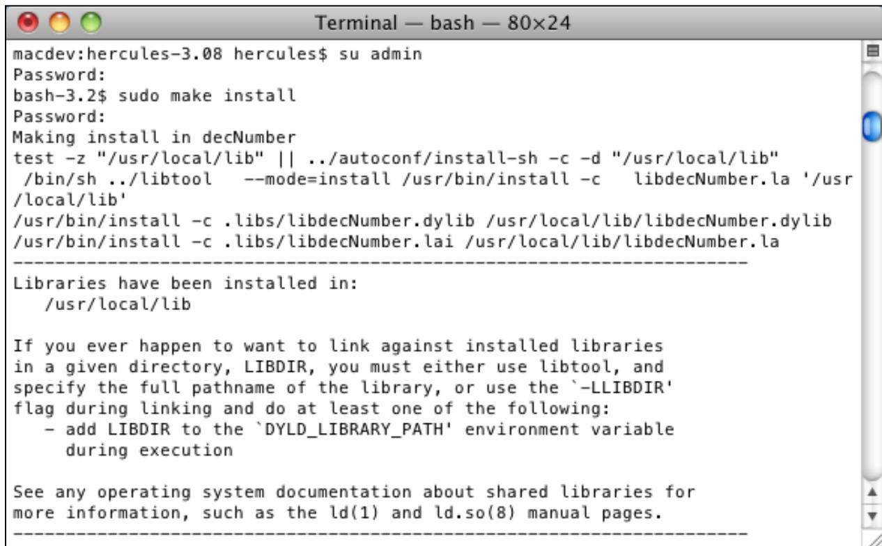
A terminal window titled "Terminal — bash — 80x24" showing the installation of the decNumber library. The user switches to the 'admin' user and runs 'sudo make install'. The output shows the installation of 'libdecNumber.dylib' and 'libdecNumber.la' to '/usr/local/lib'. It also provides instructions on how to link against these libraries using 'libtool' and the '-LLIBDIR' flag, and mentions the 'DYLD\_LIBRARY\_PATH' environment variable.
