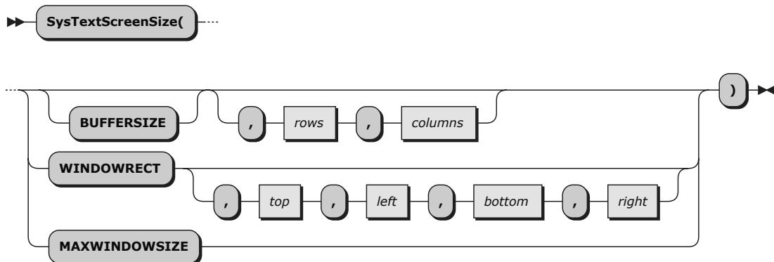
Returns or sets the size of the console screen buffer, returns or sets the position of the current console window rectangle, or returns the maximum possible console window size.
