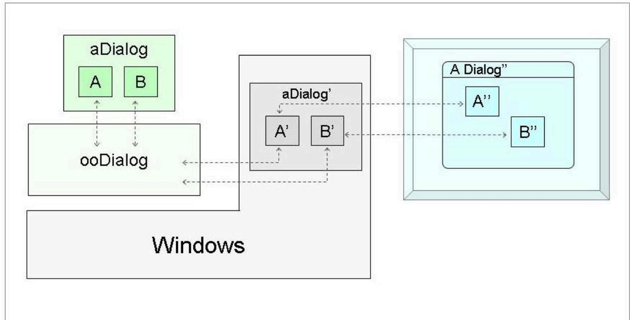
Figure 4.3. ooRexx Proxy Controls and Real Windows Controls
